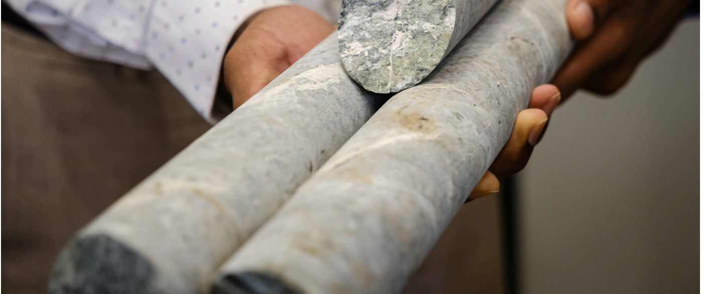
Granite rock core samples from the Sembawang drilling site. Photo from NTU
